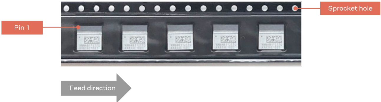
Figure 6: Orientation of ANNA-B4 modules on tape
