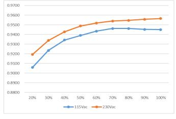
Figure 2. Typical efficiency Curve for MEU-650A24T
