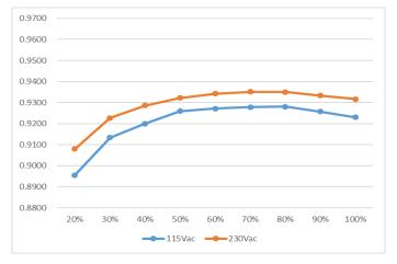
Figure 1. Typical efficiency Curve for MEU-650A12T
