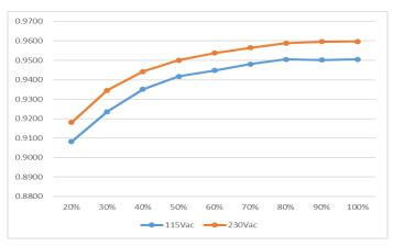
Figure 3. Typical efficiency Curve for MEU-650A48T
