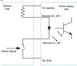
Figure 10 Remote On\_Off Connection
