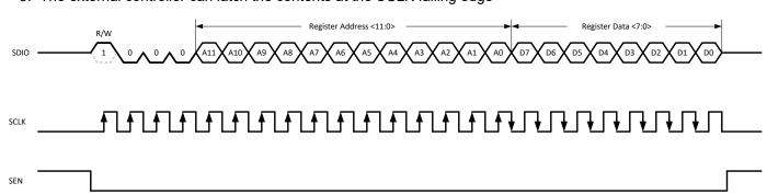
Figure 7-41. Serial Register Read Timing Diagram
