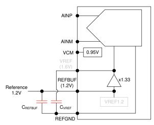
Figure 7-17. External 1.2 V reference using internal reference buffer
