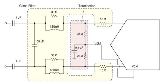
Figure 7-7. AC-Coupling: termination network provides DC bias (glitch filter example for DC - 30 MHz)
