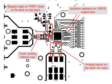
Figure 10-1. Layout example: top layer of ADC354x EVM
