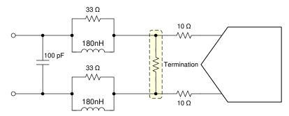
Figure 7-4. Sampling glitch filter example for input frequencies from DC to 30 MHz
