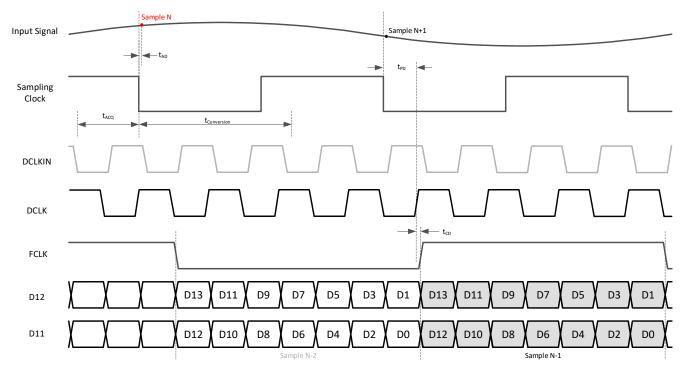
Figure 6-10. Timing Diagram: Serial CMOS 2-wire
