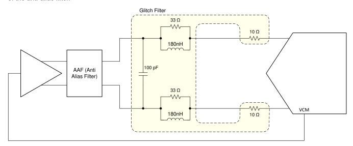
Figure 7-8. DC-Coupling: DC bias provided by FDA (glitch filter example for DC - 30 MHz)
