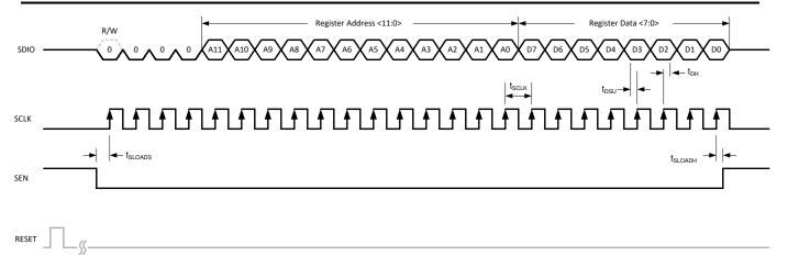
Figure 7-40. Serial Register Write Timing Diagram
