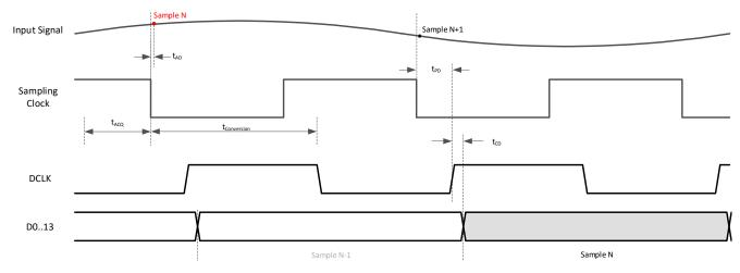
Figure 6-8. Timing Diagram: SDR CMOS
