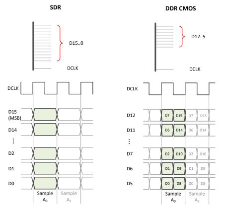
Figure 7-34. Output Data Format in Real Decimation
