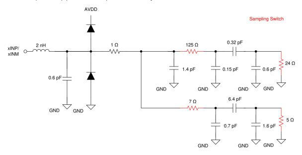
Figure 7-1. Equivalent Input Network
