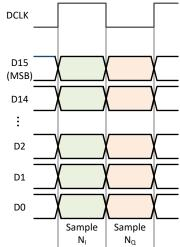
Figure 7-33. Output Data Format in Complex Decimation
