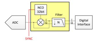
Figure 7-18. Internal Digital Decimation Filter
