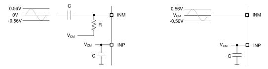
Figure 7-6. Single ended analog input: AC coupled (left) and DC coupled (right)
