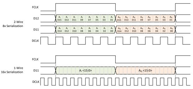
Figure 7-35. Output Data Format in Complex Decimation
