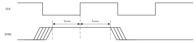
Figure 7-32. External SYNC timing diagram
