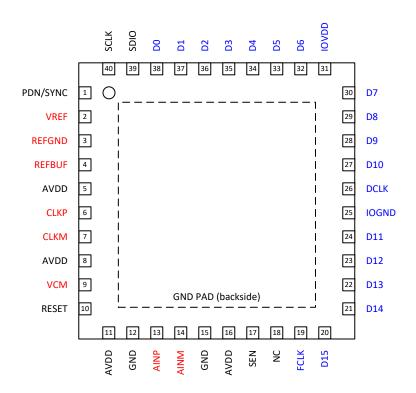
Figure 5-1. RSB Package 40-Pin WQFN Top View
