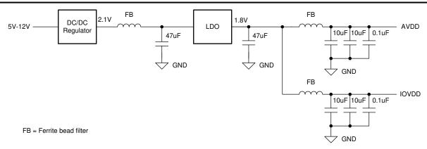
Figure 9-2. Example: LDO Linear Regulator Approach
