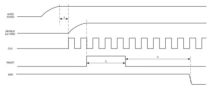
Figure 8-3. Initialization of serial registers after power up
