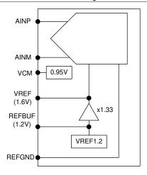
Figure 7-14. Different voltage reference options for ADC354x
