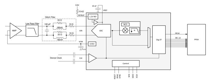
Figure 8-1. Typical configuration for a spectrum analyzer with DC support
