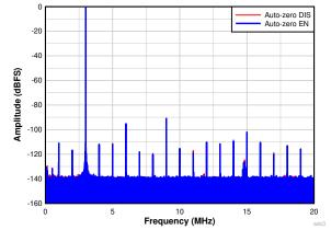
Figure 7-11. FFT at 40 MSPS with input frequency of 3 MHz (auto-zero feature enable vs disable, 4M point FFT)
