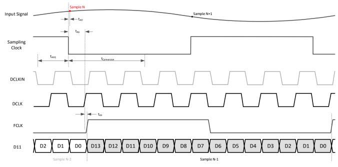
Figure 6-11. Timing Diagram: Serial CMOS 1-wire
