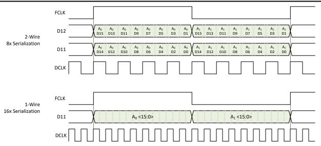
Figure 7-36. Output Data Format in Real Decimation
