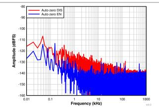
Figure 7-12. FFT at 40 MSPS with input frequency of 3 MHz (auto-zero feature enabled vs disabled, 4M point FFT)
