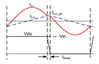
Figure 5. The primary current and voltage waveform for the LLC resonant converter
