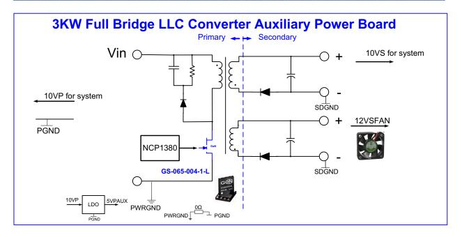
Figure 3. Auxiliary power supply block diagram for the GS-EVB-LLC-3KW-GS reference design
