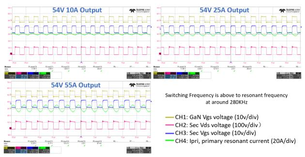
Figure 13. Steady state waveforms at 420V input and 10A, 25A, and 55A outputs
