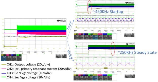
Figure 16. Full load startup waveforms at 380V, 400V, and 420V inputs
