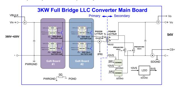
Figure 1. Simplified power stage block diagram for the GS-EVB-LLC-3KW-GS reference design
