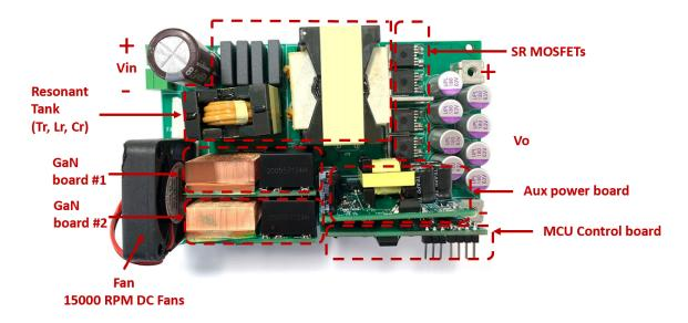
Figure 4. PCBA photos for GS-EVB-LLC-3KW-GS reference design
