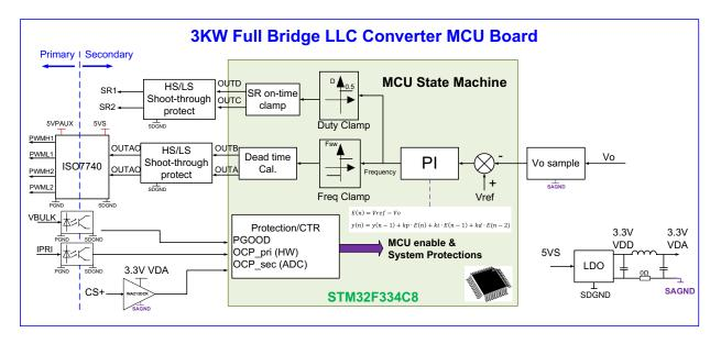
Figure 2. MCU control block diagram for the GS-EVB-LLC-3KW-GS reference design
