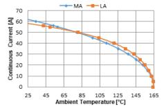
Figure 24: Maximum Continuous Current at a Given T<sub>A</sub>
