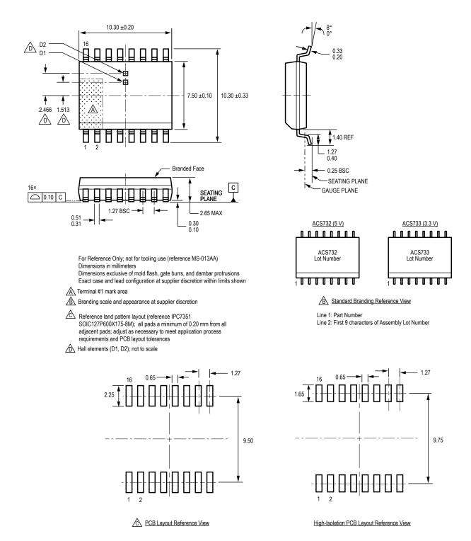
Figure 27: Package LA, 16-PIN SOICW
