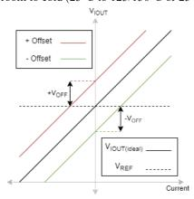
Figure 9: Offset (V<sub>OFF</sub>) Between V<sub>IOUT</sub> and V<sub>REF</sub>
