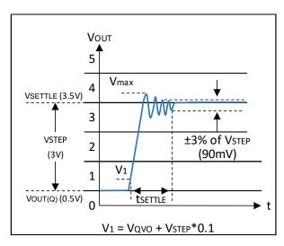
Figure 19: Overshoot and Settling Time (3 V step shown)
