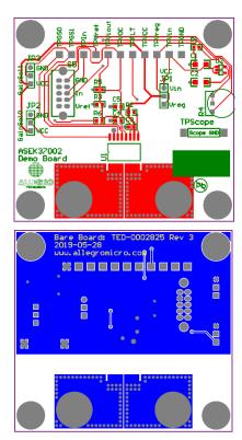
Figure 25: Top and Bottom Layers for ASEK37002
