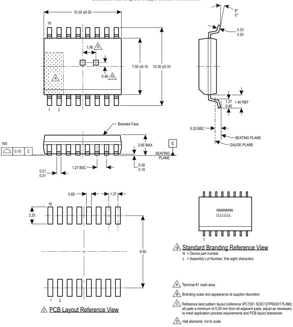
Figure 26: Package MA, 16-Pin SOICW
