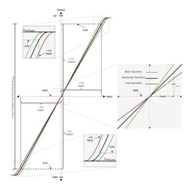
Figure 10: V<sub>OOR</sub>, V<sub>SAT</sub> and SENS with Full Scale
