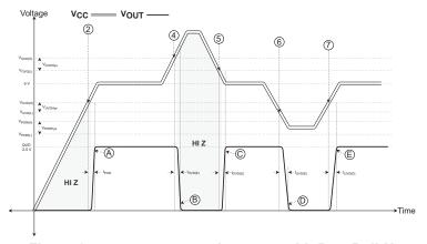
Figure 8:  $t_{POD}$ ,  $t_{OVD(E/D)}$ , and  $t_{UVD(E/D)}$  with  $R_L$  = Pull-Up
