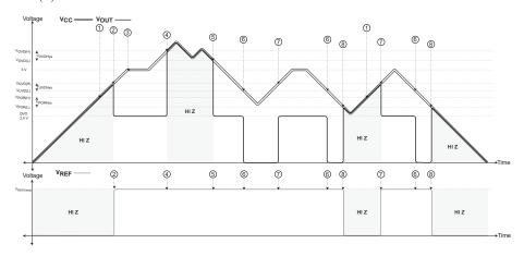
Figure 6: Power States Thresholds with  $V_{IOUT}$  and  $V_{REF}$  Behavior, 5 V Device,  $R_L$  = Pull-Up, UVD Enabled
