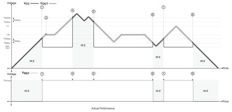
Figure 7: Power States Thresholds with  $V_{IOUT}$  and  $V_{REF}$  Behavior, 3.3 V Device,  $R_L$  = Pull-Up, UVD Disabled
