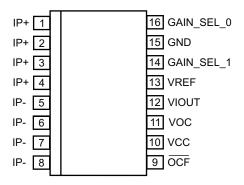
Figure 2: MA/LA Pinout Diagram
