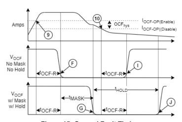
Figure 15: General Fault Timing.
