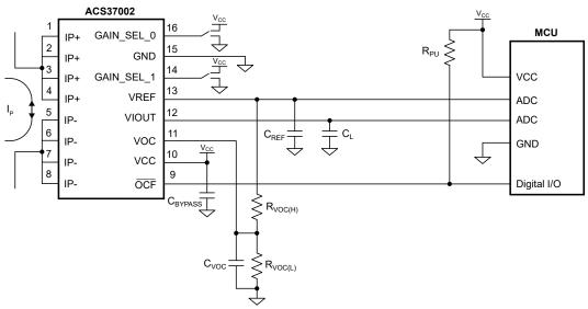
Figure 1: Typical Bidirectional Application.
