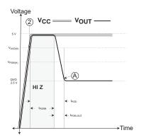
Figure 5: t<sub>POD</sub> behavior UVD disabled, RL = Pull-Up POWER-ON RESET (POR)
