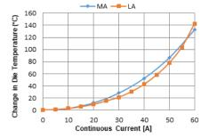
Figure 23: Self heating in the MA and LA package due to current flow
