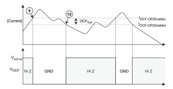
Figure 13: Fault Thresholds and OCF Pin Functionality
