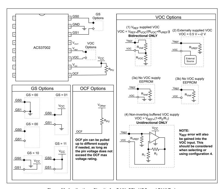
Figure 20: Applications Circuits for GAIN\_SEL, VOC, and FAULT pin
