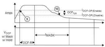
Figure 16: Fault Condition Clearing
